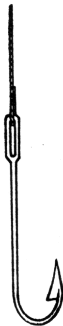
HOOK MADE OF NAIL OR TIN-CAN KEY
